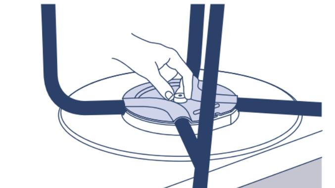
Place the lock on top of the legs, then firmly tighten the bolt in by hand.
