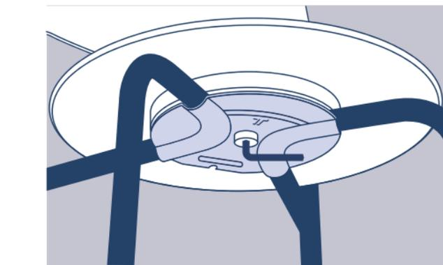
Tighten the bolt onto the lock with the Allen key one last time.
